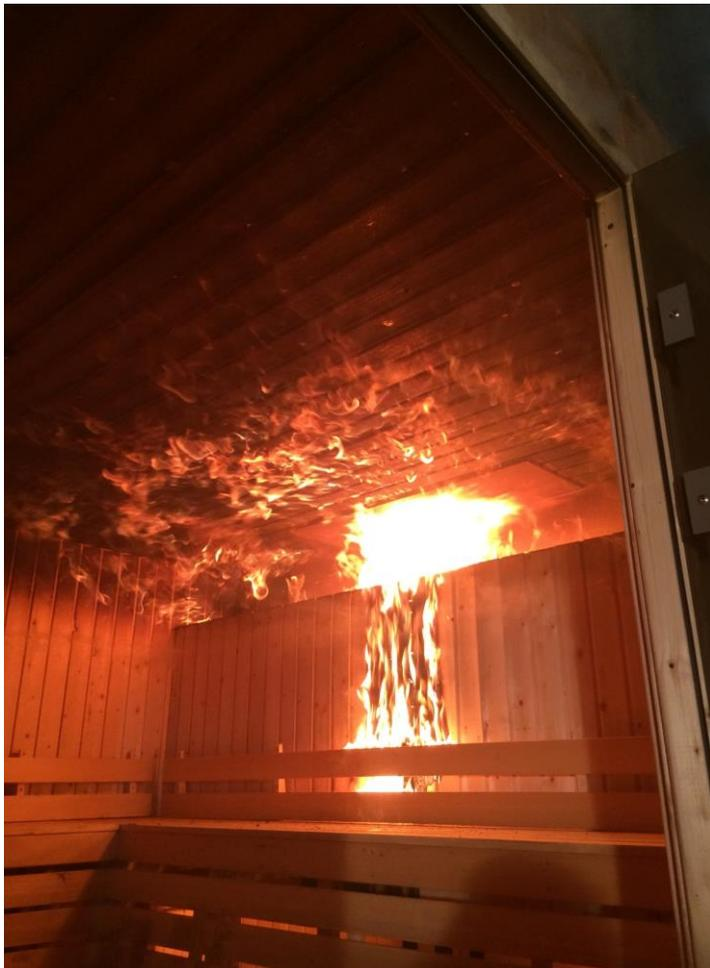
Figure 2: Flashover occurring as a result of an uncontrolled sauna fire.
